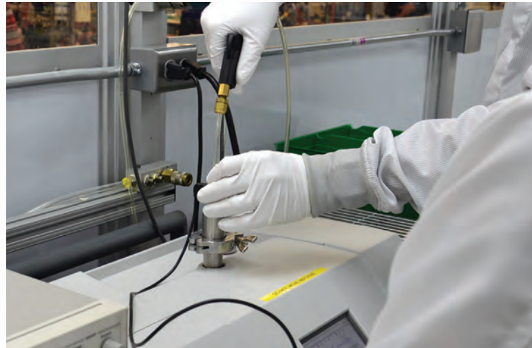
ABOVE: Performing helium leak detection test; BELOW: Custom testing station
